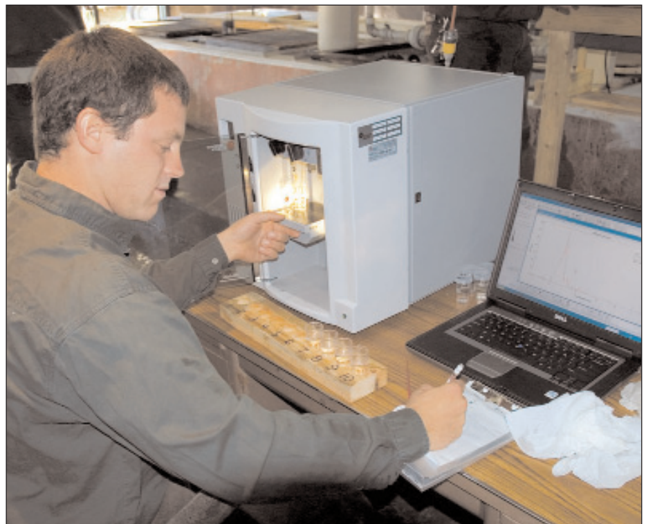
This high-tech coulter counter measures the size of each fish’s white blood cell nuclei. The nucleus of a triploid fish is 33 percent larger than that of a diploid hybrid.
